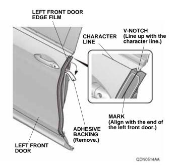
6. Line up the mark on the left front door edge film with the end of the left front door. While applying light pressure, carefully remove the adhesive backing. Go to step 10.
