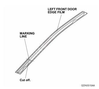
Open the left front door again. Peel back about 50 mm (1.97 in.) of adhesive backing from the left front door edge film. Line up the V-notch in the left front door edge film with the character line of the left front door.
