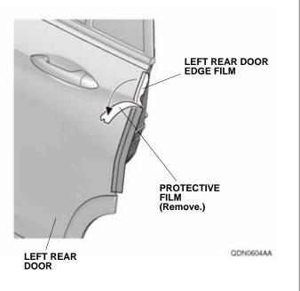
19. Starting from the center and working outward, use your fingers to fold the left rear door edge film around the edge of the left rear door. Move your fingers in one direction. Attach the left rear door edge film over the seam sealant. Do not trim or damage the seam sealant.
