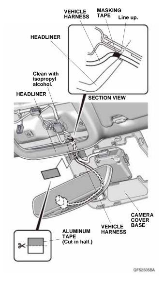
11. Using scissors, cut one aluminum tape in half. Line up the masking tape on the vehicle harness with the edge of the headliner, and secure the vehicle harness to the camera cover base with one half of aluminum tape.
