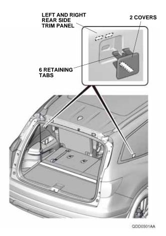
3. Install the cargo cover into the recess in the right rear side trim panel, then compress the cargo cover, and install it in the left rear side trim panel.
