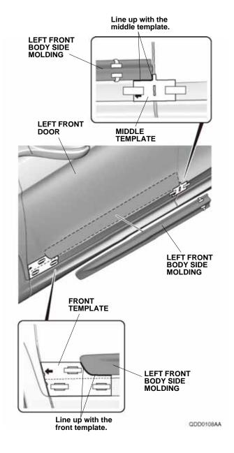
8. While applying light pressure against the left front body side molding, carefully remove the taped adhesive backings.
