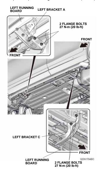
6. Repeat steps 1 through 5 on the right side of the vehicle to install the right running board.
