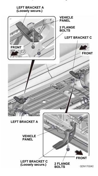
4. Secure the left running board to the left bracket A and left bracket C with four flange bolts. Torque the flange bolts to 27 N·m (20 lb·ft).
