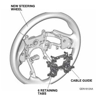
30. Install the new cable reel cord on the cable guide with one washer-screw. Plug the new cable reel cord 4-pin connector into the new steering wheel 4-pin connector, and secure the new cable reel cord to the cable guide.
