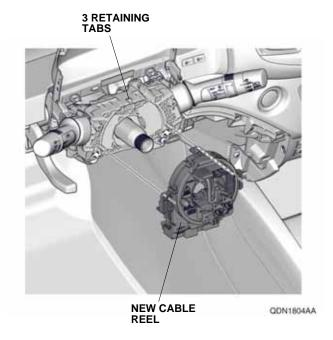
22. Plug the vehicle connectors into the new cable reel.
