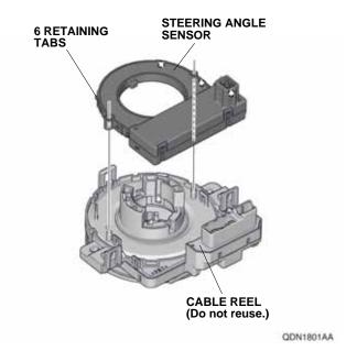
19. Install the steering angle sensor to the new cable reel with six retaining tabs.
