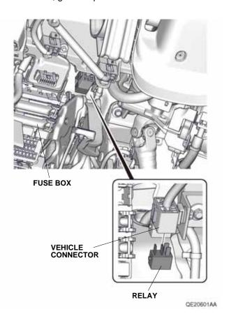
45. Install a 10 amp fuse in the #27 slot of the passenger side under hood fuse box.
