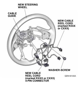
31. If equipped, install the left and right paddle shifters with two screws. Plug the new cable reel cord 4-pin connectors into the paddle shifter connectors, and secure the 4-pin connectors and paddle shifter cords on the cable guide.
