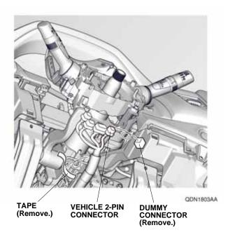
21. Install the new cable reel with three retaining tabs.
