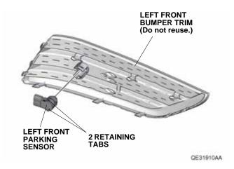
5. Install the left front parking sensor removed from step 4 into the left front bumper chrome trim.
