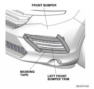
Using a plastic trim tool wrapped with the masking tape, remove the left front bumper trim and unplug the vehicle connector.
