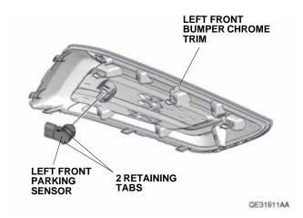
6. Plug the vehicle connector into the left front parking sensor.
