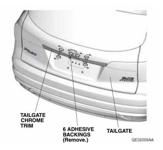
5. Using a rubber roller, apply firm pressure against the tailgate chrome trim and roll from one end to the other. Apply firm pressure especially at the ends.
