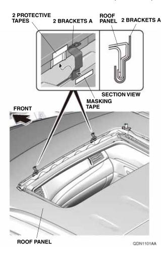
10. Set the moonroof visor on the vehicle roof in front of the moonroof opening, and adjust its position so the holes in the moonroof visor are aligned with the bracket A holes. Loosely install the moonroof visor to the brackets A with two screws and two nuts. Remove the strips of masking tape from the brackets A.
