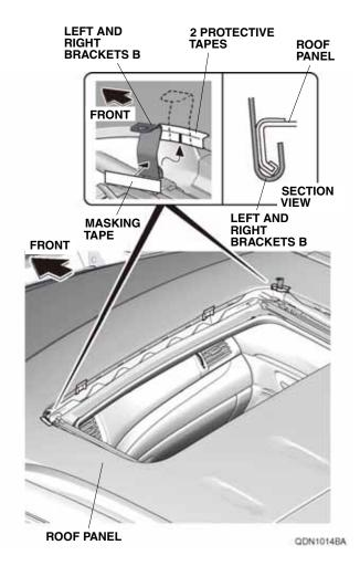
9. Place the two brackets A into position over the two protective tapes and around the lip of the roof panel, and tape them into position with strips of masking tape. Be sure to align the lower end of the brackets A with the second indentation.
