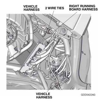
41. Bundle up the excess right running board harness, and secure it to the vehicle harness with one wire tie.
