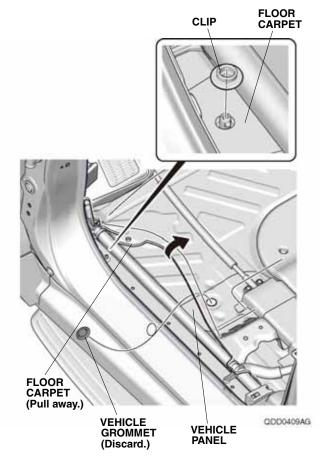
19. Locate the vehicle grommet, and remove it from the vehicle panel.
