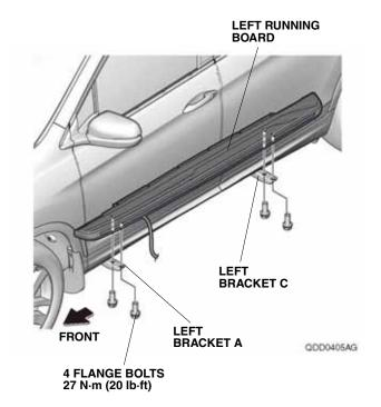
13. Tighten the four flange bolts loosely installed in step 11. Torque the flange bolts to 27 N·m (20 lb·ft).
