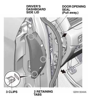
Remove the driver's dashboard lower cover, unplug the vehicle connectors, and release the vehicle sensor.
