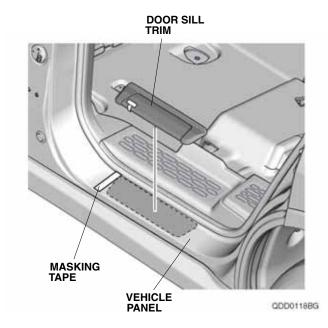
45. While applying light pressure against the door sill trim, carefully remove the adhesive backing.
