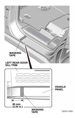
42. Using an alcohol swab, thoroughly clean the vehicle panel where the door sill trim will attach.
