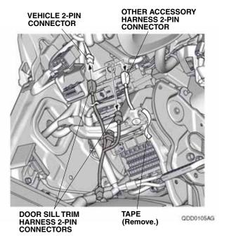
25. Remove the tape from the door sill trim harness, and plug the remaining other accessory harness 2-pin connector into the door sill trim harness 2-pin connector. Go to step 27.
