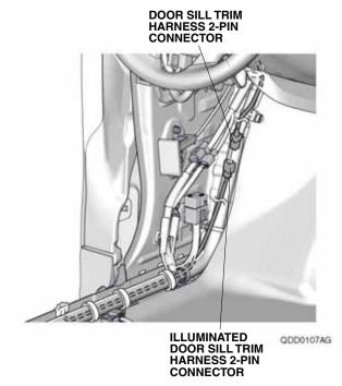
29. Bundle up the excess door sill trim harness and illuminated door sill trim harness, and secure them and 2-pin connectors to the vehicle harness with three wire ties.
