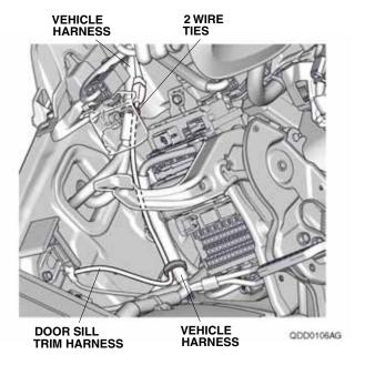
28. Plug the door sill trim harness 2-pin connector into the illuminated door sill trim harness 2-pin connector.
