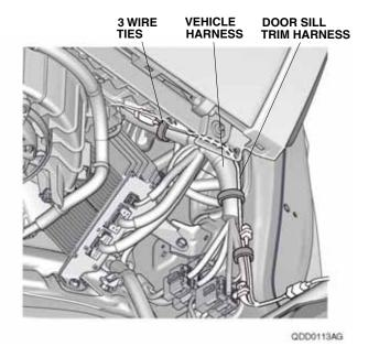
40. Secure the 2-pin connectors to the vehicle harness with one wire tie.
