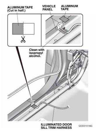
Using scissors, cut one aluminum tape in half.
