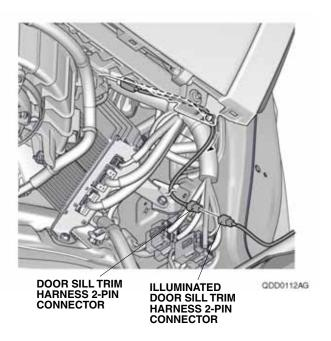
39. Secure the door sill trim harness into the vehicle harness with three wire ties.
