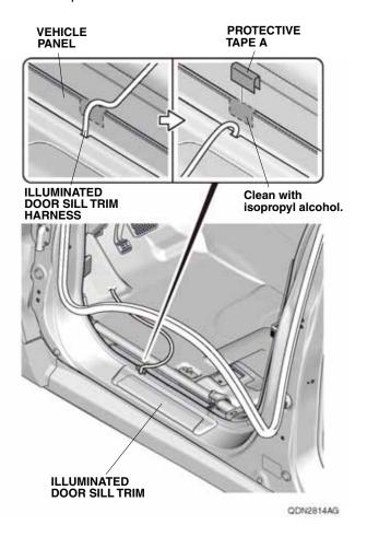
15. Install the protective clip to the protective tape A on the vehicle panel.
