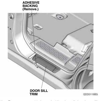
46. Repeat steps 41 through 45 to install the door sill trim on the right side of the vehicle.
