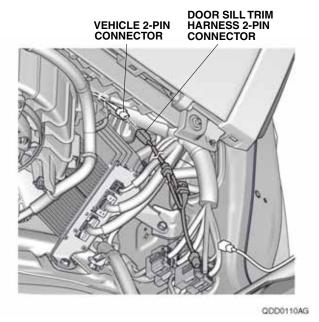
38. Plug the door sill trim harness 2-pin connector into the illuminated door sill trim harness 2-pin connector.
