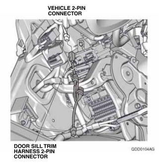
27. Secure the door sill trim harness to the vehicle harness with two wire ties.
