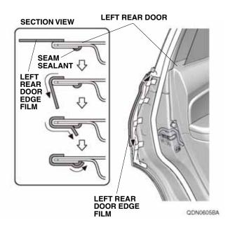
20. Using a shop towel, wipe the 3M protective tape application solution from the left rear door edge film. Allow the left rear door edge film to dry thoroughly.
