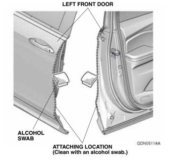
Close the left front and rear doors. Using a spray bottle with 3M protective tape application solution, spray the area where the left front door edge film will attach.
