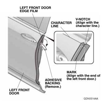
6. Align the mark on the left front door edge film with the end of the left front door. While applying light pressure, carefully remove the adhesive backing. Go to step 10.
