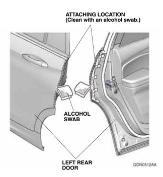
3. Open the left front door. Using an alcohol swab, thoroughly clean the area where the left front door edge film will attach.
