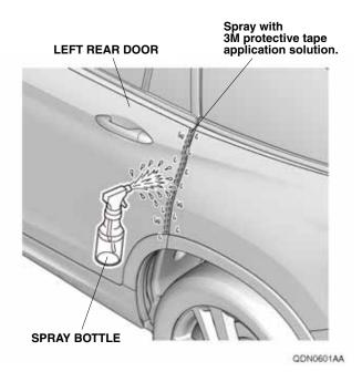
Open the left rear door again. Peel back about 50 mm (1.97 in.) of adhesive backing from the left rear door edge film. Align the V-notch in the left rear door edge film with the character line of the left rear door.
