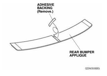
4. Align the center of the rear bumper applique with the mark on the masking tape. Align the front edge of the applique along the edge of the curved surface as shown. Attach the center of the rear bumper applique to the rear bumper.
