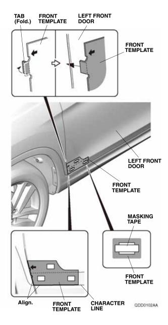
2. Align the middle template with the character line, and attach it to the left front door and left rear door with strips of masking tape as shown.
