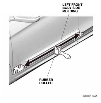
Peel back the adhesive backings, and tape them to the front surface of the left rear body side molding with the strips of masking tape. Remove the small piece of adhesive backings.
