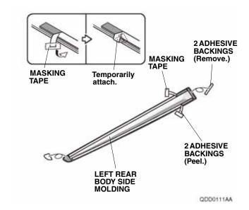
11. Align the left rear body side molding with the middle and rear templates, and attach it to the left rear door as shown.
