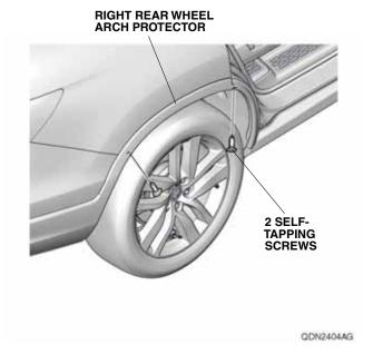
17. Remove the two self-tapping screws from the right rear wheel arch protector.
