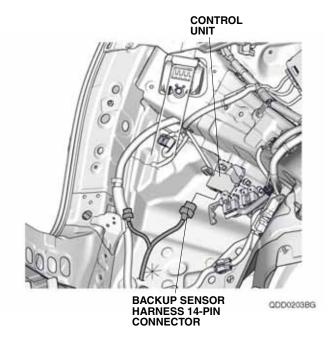
If the vehicle is equipped with the trailer hitch harness, continue with step 27; otherwise, go to step 30.
