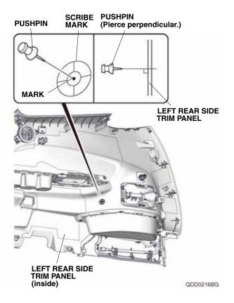
41. While wearing eye protection, drill the pierced mark on the left rear side trim panel with a 3 mm drill bit. Enlarge the 3 mm hole to 26 mm using a 26 mm hole saw. Remove any burrs.
