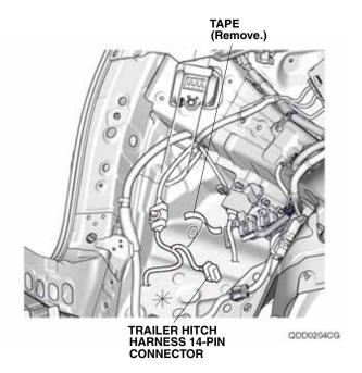
28. Plug the trailer hitch harness 14-pin connector into the backup sensor harness 14-pin connector.
