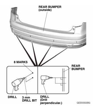
53. While wearing eye protection and drilling from painted side of the rear bumper, enlarge the left lower 3 mm outer hole and right upper 3 mm outer hole to 24 mm using a 24 mm hole saw.
