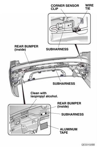
62. Secure the subharness to the rear bumper and corner sensor clip with one aluminum tape and one wire tie as shown.
