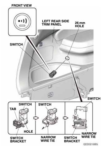
43. Align the tab on the switch bracket with the hole in the switch and secure the switch bracket to the switch with one narrow wire tie.
