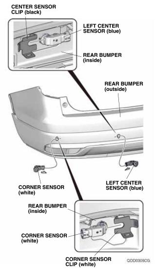
56. Secure the corner sensor (white) and left center sensor (blue) with corner sensor clip (white) and center sensor clip (black) as shown.
