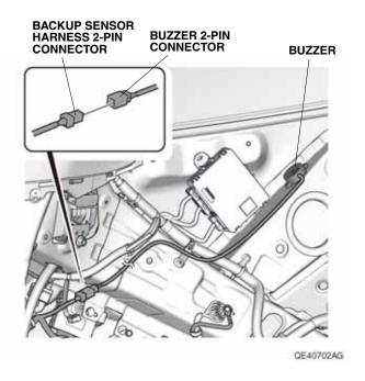
39. Bundle up the excess buzzer harness, and secure the buzzer harness and 2-pin connectors to the vehicle harness with three wire ties.
