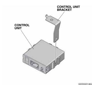
25. Insert the control unit bracket into the hole in the vehicle panel, and secure it with one flange bolt.
