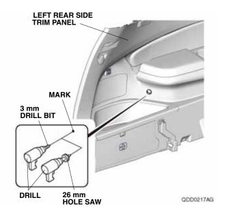
42. Install the switch into the 26 mm hole in the left rear side trim panel.
