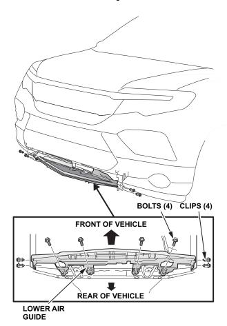
5. Remove the front bumper center lower grille NOTE: If equipped, remove the parking sensor sub harness clamps.
