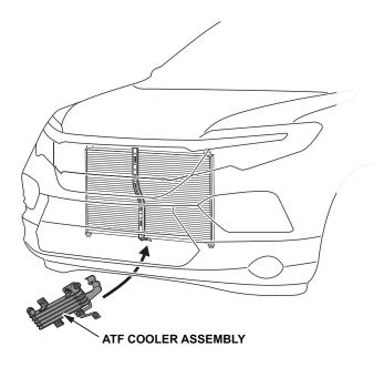
Install the ATF cooler with three 6 x 20 mm washer bolts.
