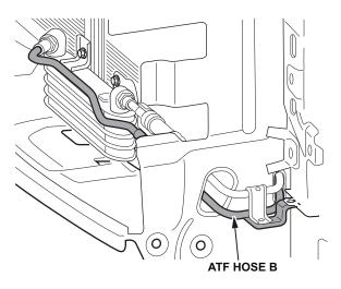
Install the hose bracket using a 6 x 16 mm washer bolt.
