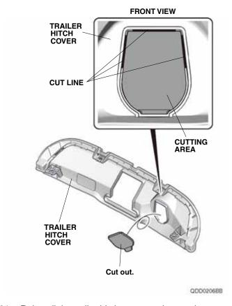
21. Reinstall the trailer hitch cover on the rear bumper.
