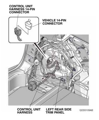
9. Secure the 14-pin connectors to the back of the left rear side trim panel with the clip on the control unit harness 14-pin connector.
