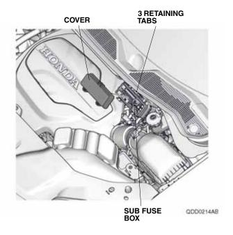
33. Plug the two 20A blade fuses and the 30A block fuse into the sub fuse box.
