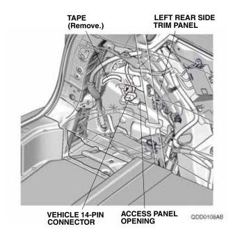
8. Route the control unit harness 14-pin connector and plug it into the vehicle 14-pin connector.
