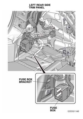
29. Install the two relays into the fuse box on the control unit harness.
