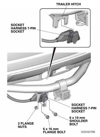
23. Refer to the trailer hitch installation instructions, reinstall the trailer hitch.
