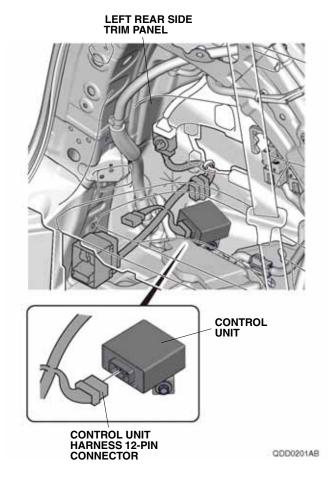
14. Install the control unit on the vehicle panel as shown.
