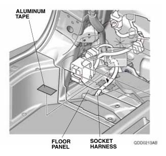
31. Secure the socket harness to the floor panel with one aluminum tape.
