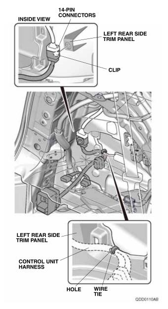
10. Secure the control unit harness to the left rear side trim panel with one wire tie.
