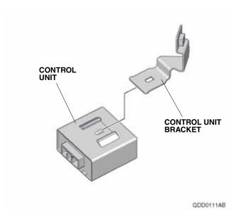
12. Loosely install the washer-bolt on the control unit bracket.
