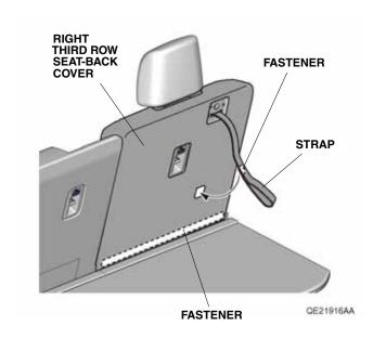
6. Install the left third row seat-back cover to the left third row seat-back. Pull the strap through the hole on the left third row seat-back cover.
