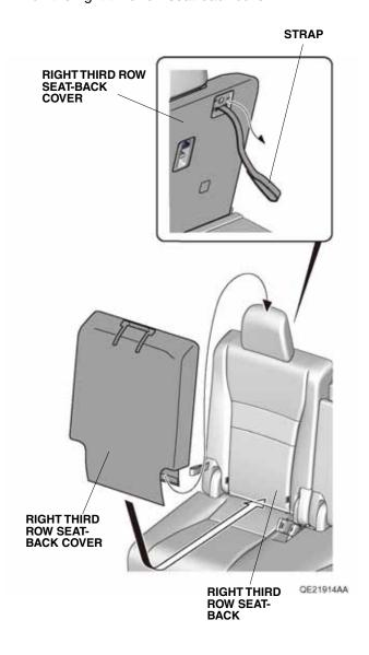
Secure the right third row seat-back cover with the fasteners.
