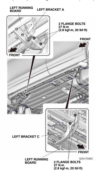
6. Repeat steps 1 through 5 on the right side of the vehicle to install the right running board.
