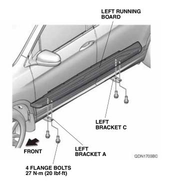
5. Tighten the four flange bolts loosely installed in step 3. Torque the flange bolts to 27 N·m (20 lbf·ft).
