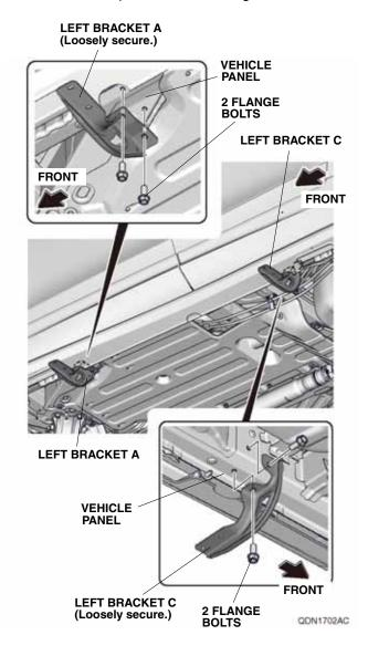
4. Secure the left running board to the left bracket A and left bracket C with four flange bolts. Torque the flange bolts to 27 N·m (20 lbf·ft).
