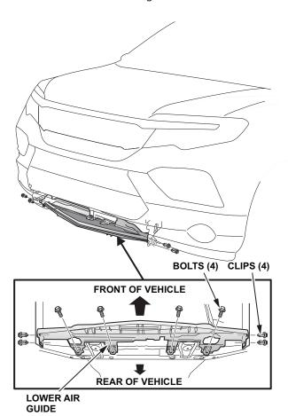
4. Remove the front bumper center lower grille NOTE: If equipped, remove the parking sensor sub harness clamps.
