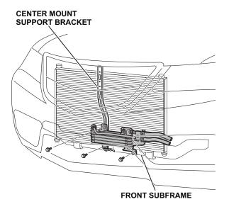
7. Install the ATF pipe assembly bracket to the vehicle's frame with the 6 x 12 mm flange bolt.
