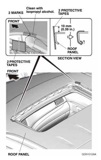
Remove the adhesive backing from the two protective tapes, and attach one to the roof panel at each of the two marks you made.
