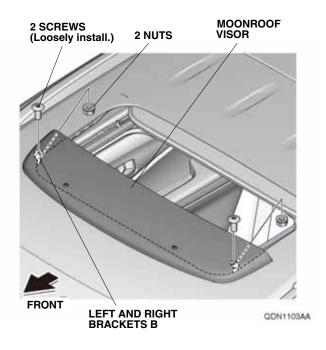
12. Position the moonroof visor with equal spacing on each side. Check that the rubber molding is not twisted or rolled under the moonroof visor.
