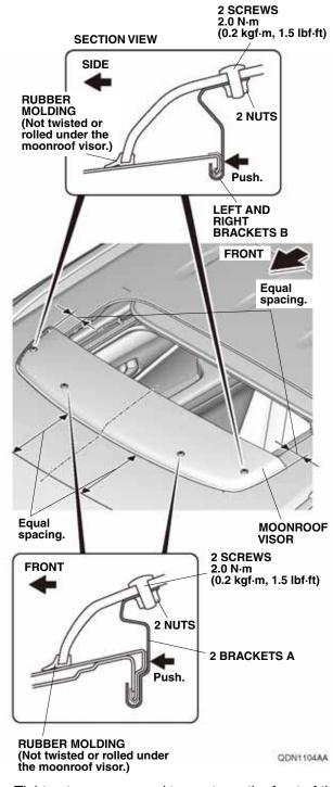
Tighten two screws and two nuts on the front of the vehicle first, then tighten two screws and two nuts on each side. Tighten while applying pressure so that there is no gap between the roof panel and the brackets A and B. Torque the screws to 2.0 N·m (1.5 lbf·ft).
