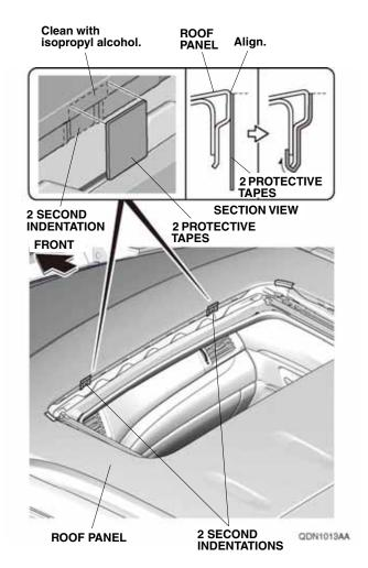
7. Remove the adhesive backing from the two protective tapes, and attach one to the roof panel at each second indentation.
