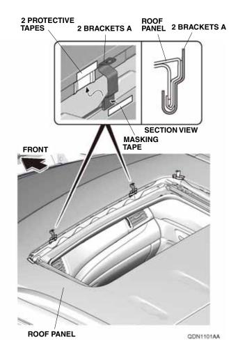
Set the moonroof visor on the vehicle roof in front of the moonroof opening, and adjust its position so the holes in the moonroof visor are aligned with the bracket A holes. Loosely install the moonroof visor to the brackets A with two screws and two nuts. Remove the strips of masking tape from the brackets A.
