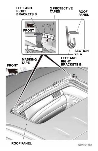
9. Place the two brackets A into position over the two protective tapes and around the lip of the roof panel, and tape them into position with masking tape. Be sure to align the lower end of the brackets A with the second indentation.
