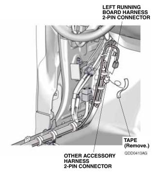
26. Bundle up the excess left running board harness, and secure it to the vehicle harness with two wire ties. Go to step 30.
