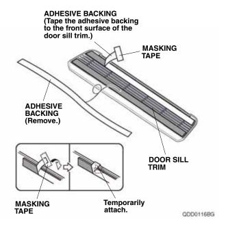
44. Align the door sill trim with the masking tape and install the door sill trim to the vehicle panel.
