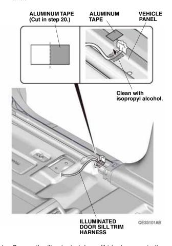
31. Secure the illuminated door sill trim harness to the vehicle panel with one piece of aluminum tape cut in step 20.
