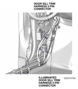
29. Bundle up the excess door sill trim harness and illuminated door sill trim harness, and secure them and 2-pin connectors to the vehicle harness with three wire ties.
