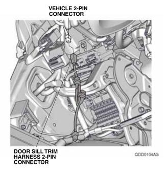
27. Secure the door sill trim harness to the vehicle harness with two wire ties.
