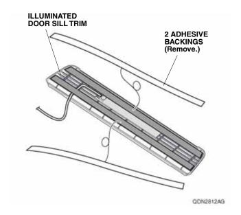
13. Align the cutout shape on the illuminated door sill trim with the bump shape on the vehicle panel. Press on the adhesive part of the illuminated door sill trim firmly.
