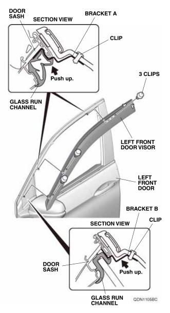
Secure the left front door visor to two brackets A and one bracket B with three clips. Make sure to push up on the two brackets A and one bracket B while installing the clips.
