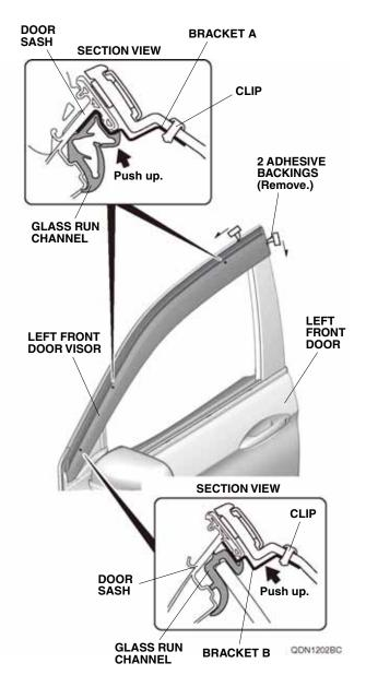
12. Using the palm of your hand, firmly press the left front door visor against the door sash.
