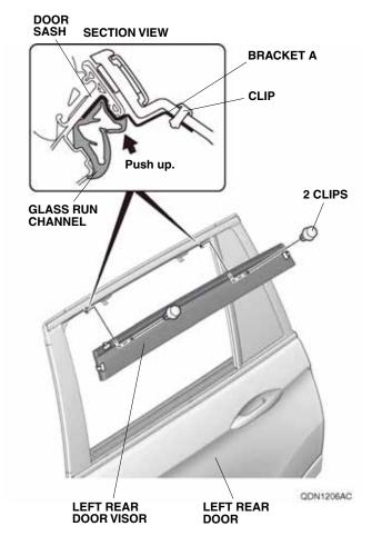
20. Secure the left rear door visor to two brackets A with two clips. Make sure to push up on the two brackets A while installing two clips. NOTE: The clips cannot be removed and reinstalled after installation.
