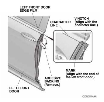
Align the mark on the left front door edge film with the end of the left front door. While applying light pressure, carefully remove the adhesive backing. Go to step 10.
