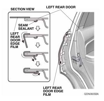
20. Using a shop towel, wipe the 3M protective tape application solution from the left rear door edge film. Allow the left rear door edge film to dry thoroughly.
