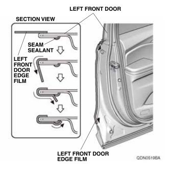
Using a shop towel, wipe the 3M protective tape application solution from the left front door edge film. Allow the left front door edge film to dry thoroughly.
