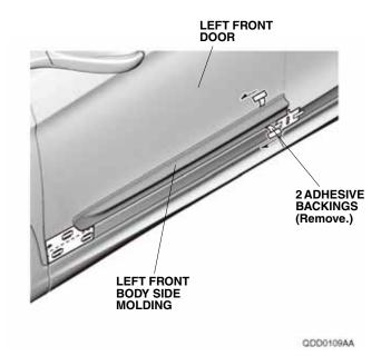
9. Using a rubber roller, apply firm pressure against the left front body side molding and roll from one end to the other. Apply firm pressure especially at the ends.
