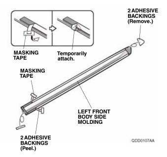
7. Align the left front body side molding with the front and middle templates, and attach it to the left front door as shown.
