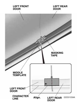
3. Align the rear template with the character line, and attach it to the left rear door with strips of masking tape as shown.
