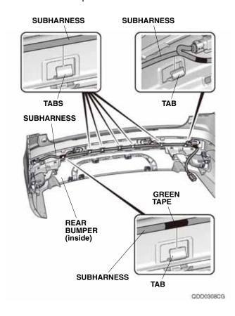
61. Using isopropyl alcohol on a shop towel, thoroughly clean the rear bumper where the aluminum tape will attach.
