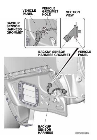
Secure the backup sensor harness 8-pin connector to the vehicle harness with one wire tie with holder.
