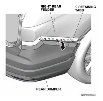
On each side, release the two retaining tabs.
