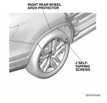
17. Remove the two self-tapping screws from the right rear wheel arch protector.
