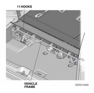
7. Remove the vehicle frame from the left and right rear side trim panel.
