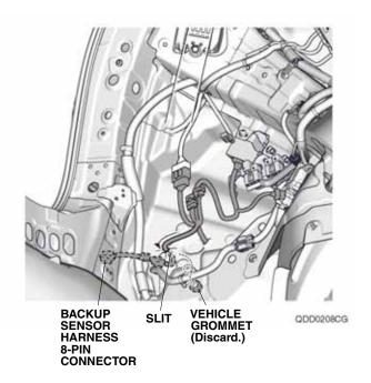
32. Secure the backup sensor harness grommet into the vehicle grommet hole.
