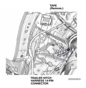
28. Plug the trailer hitch harness 14-pin connector into the backup sensor harness 14-pin connector.
