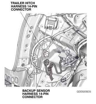
Install the 14-pin connectors to the trailer hitch harness 14-pin connectors as shown. Go to step 31.
