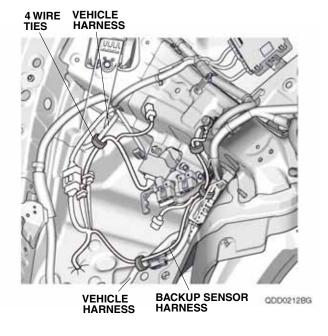
36. Using isopropyl alcohol on a shop towel, thoroughly clean the vehicle panel where the buzzer will attach.
