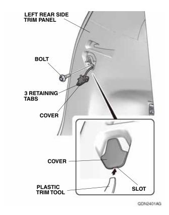
13. Pull the cover, and remove the screw.
