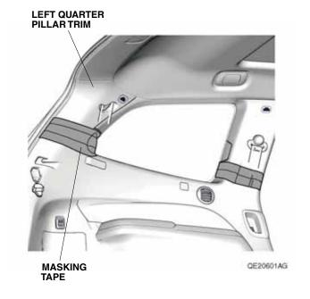
15. Remove the left rear side trim panel and unplug the vehicle connector.
