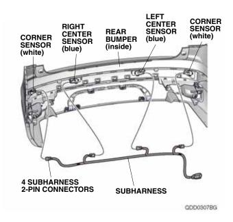
60. Align and secure the green tape on the subharness to the rear bumper as shown.
