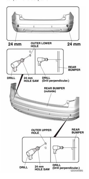
54. While wearing eye protection and drilling from painted side of the rear bumper, enlarge the two upper 3 mm inner holes to 26 mm using a 26 mm hole saw.
