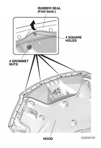
Fold back the rubber seal, and using an alcohol swab, clean the areas of the hood where the two brackets A and the two brackets B will mount.
