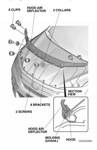
10. Open the hood. Tighten the four truss screws loosely installed in step 4.
