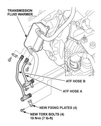
7. Make sure the connection points are clean and free of debris, then install ATF pipe A and ATF pipe B using the new fixing plates and Torx bolts supplied in this kit.
