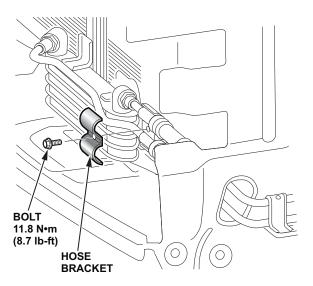
15. Secure hose A and hose B to the bulkhead using the two 6 x 12 mm washer bolts.
