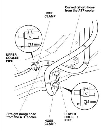
13. Remove the plug from the upper cooler pipe, and install the straight (long) hose from the ATF cooler to the upper pipe using the other supplied hose clamp.
