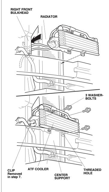
Install the clip on the power steering reservoir return hose (removed in step 7) into the clip hole in the ATF cooler.
