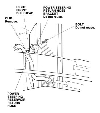
8. Remove the power steering return hose bracket (one bolt). The bolt and bracket will not be reused.
