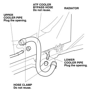
Remove the plug from the lower cooler pipe, and install the curved (short) hose from the ATF cooler to the lower pipe using one of the supplied hose clamps.
