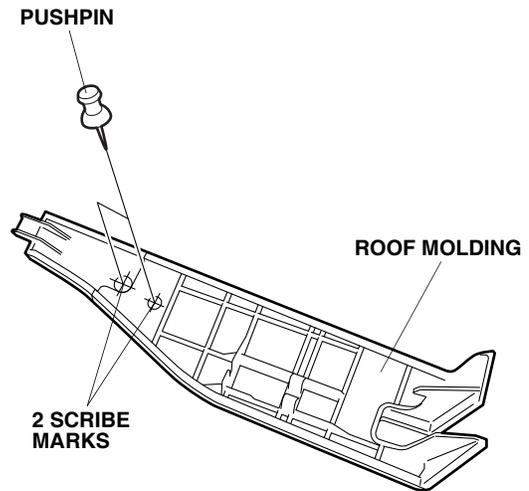
3. While wearing eye protection, drill two holes in the roof molding with a 3 mm drill bit at the holes made in step 2.
