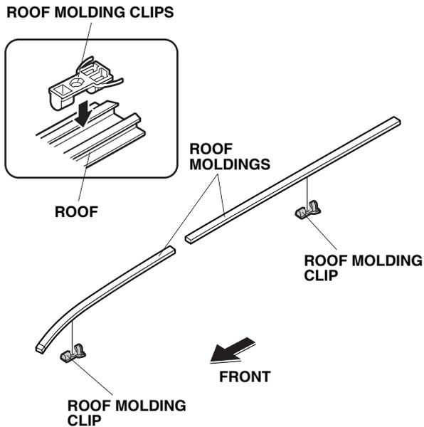
12. Reinstall the roof moldings onto the roof of the vehicle with two new roof molding clips installed in step 10.
