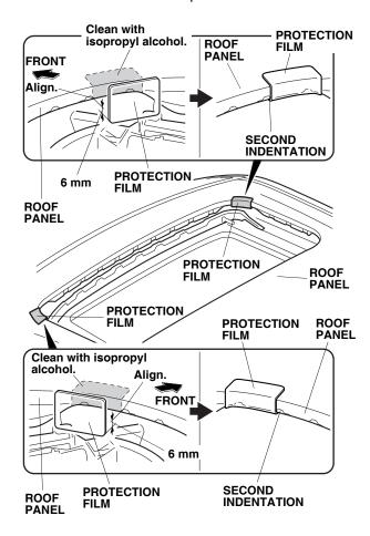
8. Remove the adhesive backings from the protection film. Starting from the bottom edge of the protection film, wrap 6 mm of the protection film around the lip of the roof panel opening and align it with the second indentation on the left side of the roof panel as shown; continue upward with the protection film around the top of the roof panel. Repeat the same procedure for the right side of the roof panel.
