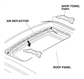
6. Roll up two shop towels and insert them between the roof panel and air deflector to lower the air deflector. Do not to damage the air deflector.
