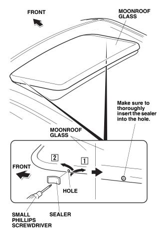
4. Insert the rest of the sealer towards the front of the hole as shown. Make sure to thoroughly insert the sealer into the hole.
