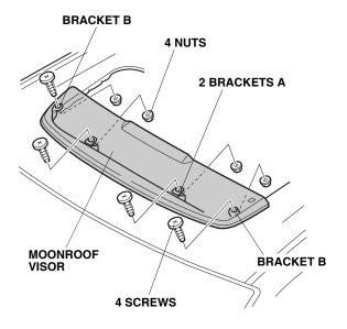
14. Adjust the position of the moonroof visor. Check that the brackets A and brackets B are firmly secured. Make sure the rubber molding on the moonroof visor is not twisted or rolled under the visor, and unfold if necessary.
