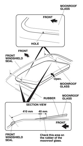
2. Measure and check the area on the rubber of the moonroof glass on the left and right side of the vehicle. If a hole is located on the rubber of the moonroof glass in the area shown, go to step 3; if not, go to step 5.
