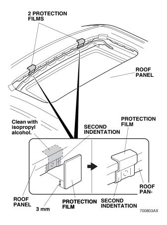
10. Remove the adhesive backings from the protection film. Starting from the bottom edge of the protection film, wrap 3 mm of the protection film around the lip of the roof panel opening to cover the second indentation on the left side of the roof panel; continue upward with the protection film around the top of the roof panel. Repeat the same procedure for the right side of the roof panel.
