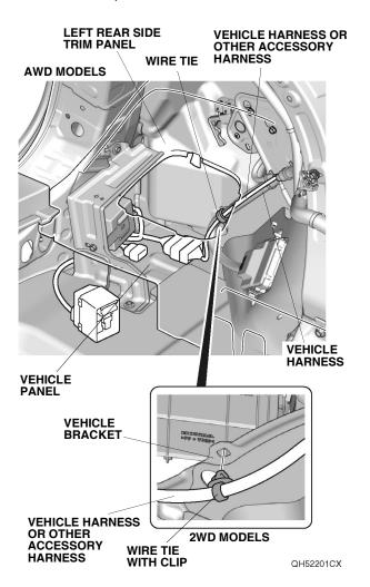
24. Using isopropyl alcohol on a shop towel, thoroughly clean the vehicle panel where the aluminum tape will attach.
