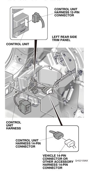
22. Plug the control unit harness 12-pin connector into the control unit. Then, plug the vehicle 14-pin connector or other accessory harness 14-pin connector into the control unit harness 14-pin connector.
