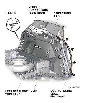
14. Release the vehicle harness to remove the left rear insulator.
