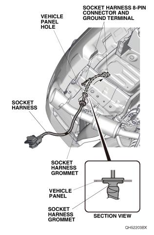
28. Route the socket harness 8-pin connector and socket harness ground terminal through the vehicle panel hole, and install the socket harness grommet into the vehicle panel hole.
