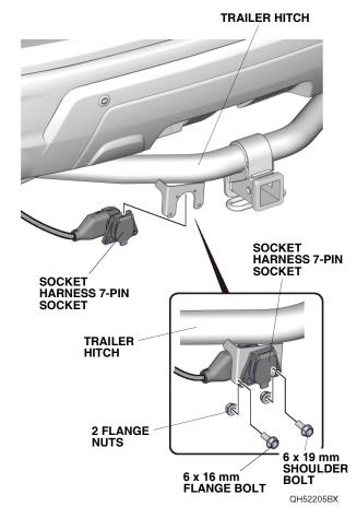
31. Refer to the installation instructions of the trailer hitch, install the trailer hitch.
