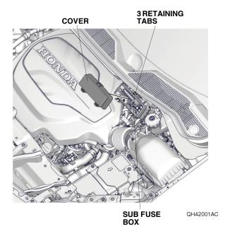
42. Plug the two 20A blade fuses and the 30A block fuse into the sub fuse box.
