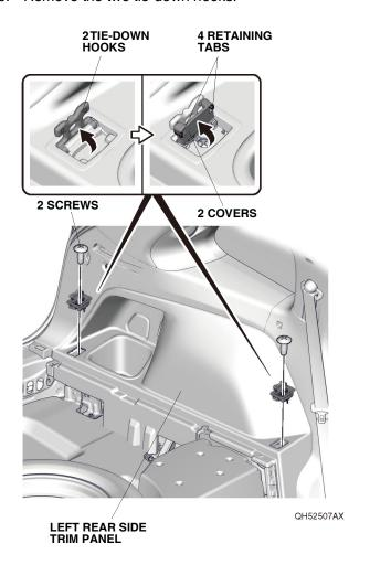
11. Using a plastic trim tool, pull the cover, and remove the cargo hook.
