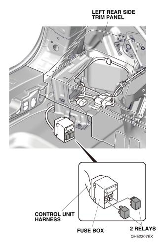
35. Secure the socket harness ground terminal and fuse box bracket to the vehicle bracket with one ground bolt.
