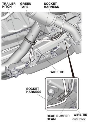
33. Secure the socket harness to the rear bumper beam with one wire tie as shown.
