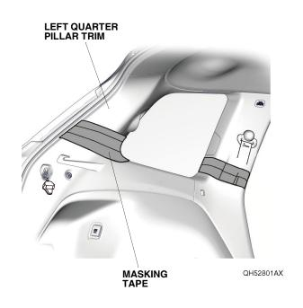
Pull away the door opening seal from around the left rear side trim panel. Remove the left rear side trim panel, and unplug the vehicle connectors (if equipped).
