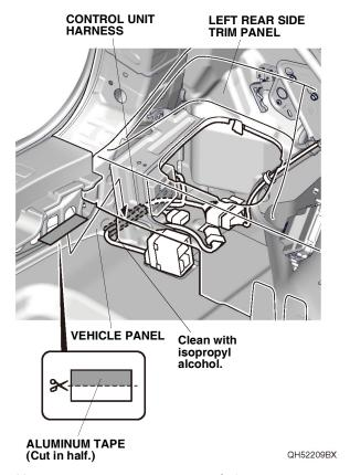
37. Using scissors, cut one piece of aluminum tape in half, and secure the control unit harness to the vehicle panel with only one piece of aluminum tape.
