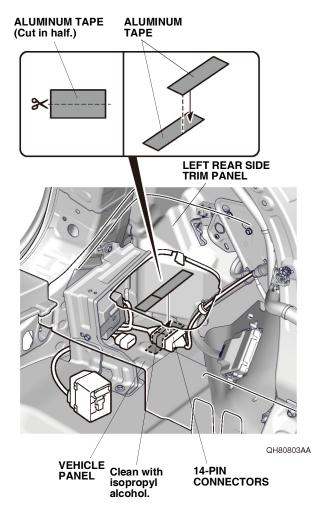
25. Using scissors, cut one piece of aluminum tape in half, and secure the 14-pin connectors to the vehicle panel with two pieces of aluminum tape as shown.
