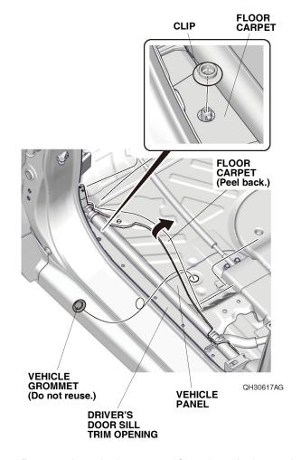
24. Remove the vehicle grommet from the vehicle panel.
