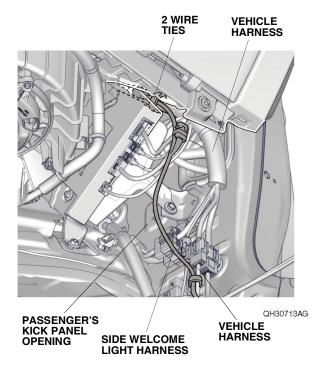
48. Bundle up the excess side welcome light harness, and secure it to the vehicle harness with one wire tie as shown. Go to step 51.
