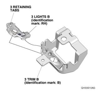
17. Install the three retainers to each trim B with three self-tapping screws as shown.
