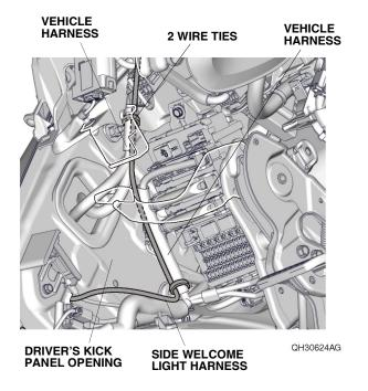
32. Secure the side welcome light harness to the vehicle harness with two wire ties. Go to step 35.
