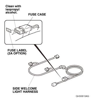
37. Plug the three side welcome light harness 2-pin connectors into the one light A and two lights B.
