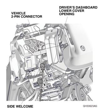
Secure the side welcome light harness to the vehicle harness with two wire ties.
