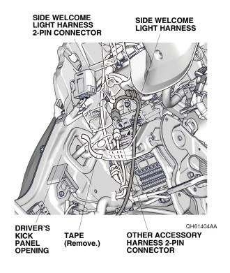
34. Bundle up the excess side welcome light harness, and secure it and 2-pin connectors to the vehicle harness with two wire ties as shown.
