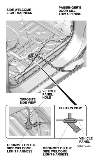
42. Secure the grommet on the side welcome light harness to the vehicle panel hole.
