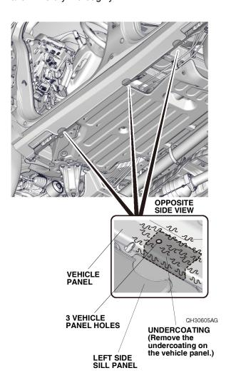
12. Using a pushpin, pierce the left side sill panel as shown.
