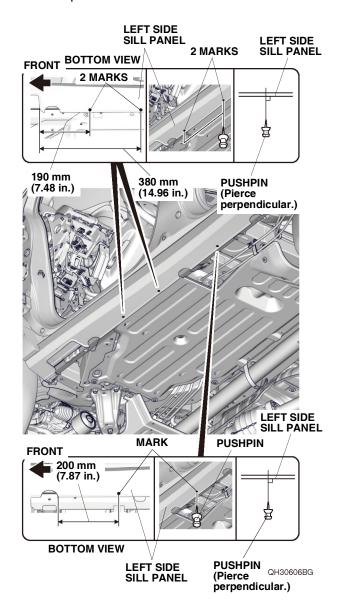
13. While wearing eye protection, drill the three pierced marks on the left side sill panel to 6 mm. First drill with a 3 mm drill bit, and finish with a 6 mm drill bit. NOTE: Make sure to drill perpendicular to the left side sill panel.
