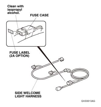
Plug the three side welcome light harness 2-pin connectors into the two lights A and one light B.
