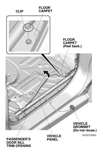
40. Remove the vehicle grommet from the vehicle panel.
