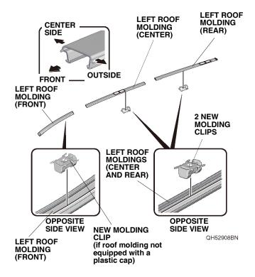
Install the left roof moldings with molding clips. Line
