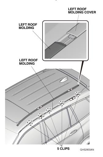
5. Remove the five clips from either the molding or the roof stud bolts.
