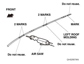
9. Install the new molding clips to the left roof moldings as shown.
