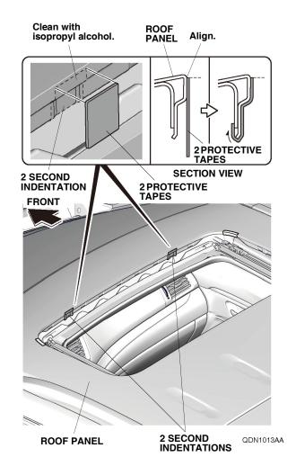
6. Remove the adhesive backing from the two protective tapes, and attach one to the roof panel at each second indentation.
