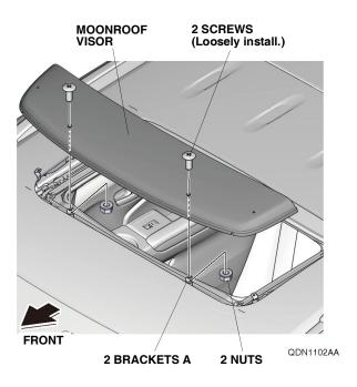
10. Loosely install the moonroof visor to the brackets B with two screws and two nuts. Remove the strips of masking tape from the brackets B.
