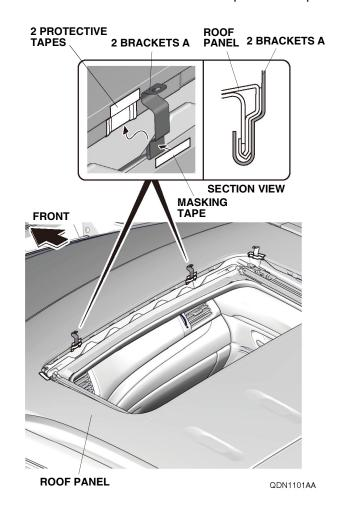
9. Set the moonroof visor on the vehicle roof in front of the moonroof opening, and adjust its position so the holes in the moonroof visor are aligned with the bracket A holes. Loosely install the moonroof visor to the brackets A with two screws and two nuts. Remove the strips of masking tape from the brackets A.
