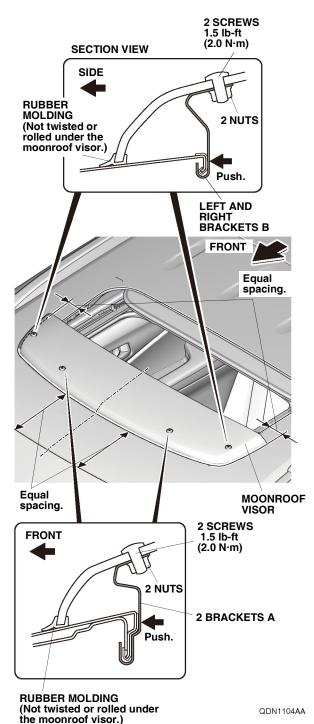
Tighten two screws and two nuts on the front of the 13. vehicle first, then tighten two screws and two nuts on each side. Tighten while applying pressure so that there is no gap between the roof panel and the brackets A and B. Torgue the screws to 1.5 lb-ft (2.0 N·m).
