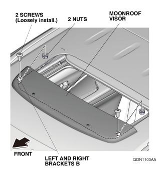
11. Check the information of the IMPORTANT INFORMATION label. To avoid wind noise, install the brackets against the body.
