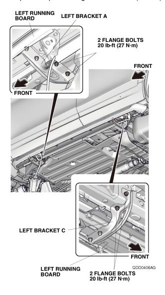
14. Line up the green tape on the left running board harness with the hole on the left bracket A, and secure the left running board harness to the left bracket A with one wire tie.
