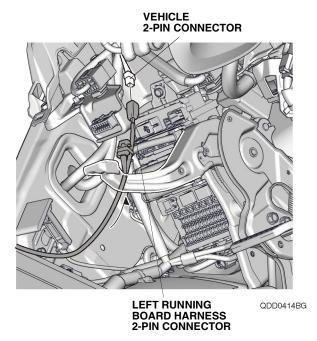
28. Secure the left running board harness to the vehicle harness with two wire ties.
