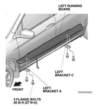
13. Tighten the four flange bolts loosely installed in step 11. Torque the flange bolts to 20 lb-ft (27 N·m).
