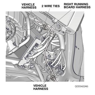
Bundle up the excess right running board harness, and secure it to the vehicle harness with one wire tie.
