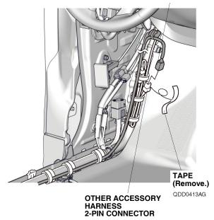
26. Bundle up the excess left running board harness, and secure it to the vehicle harness with two wire ties. Go to step 30.
