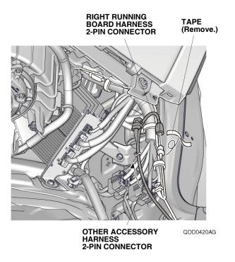
38. Bundle up the excess right running board harness, and secure it to the vehicle harness with two wire ties. Go to step 41.
