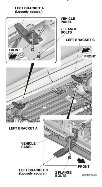
12. Secure the left running board to the left bracket A and left bracket C with four flange bolts. Torque the flange bolts to 20 lb-ft (27 N·m).
