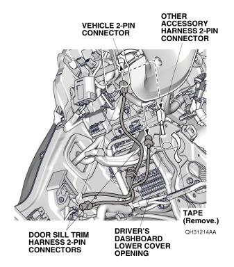
41. Remove the tape to free the door sill trim harness 2-pin connector, and plug it into the other accessory harness 2-pin connector. Go to step 43.
