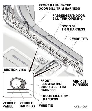
72. Plug the door sill trim harness 2-pin connector into the front illuminated door sill trim harness 2-pin connector, and secure the 2-pin connectors and door sill trim harness to the vehicle harness with one wire tie.
