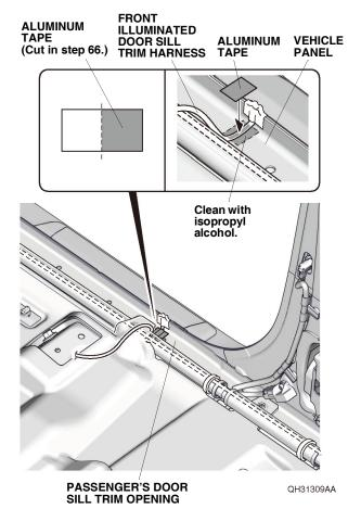
Secure the front illuminated door sill trim harness to the vehicle panel with one piece of aluminum tape cut in step 66.
