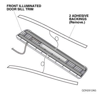
22. Line up the cutout shape on the front illuminated door sill trim with the bump shape on the vehicle panel. Press down firmly on the adhesive part of the front illuminated door sill trim firmly.
