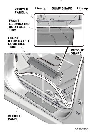
23. Using isopropyl alcohol on a shop towel, thoroughly clean the vehicle panel where the protective tape will attach. Attach one protective tape A to the vehicle panel as shown.
