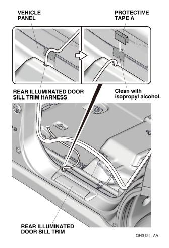
35. Install the protective clip to the protective tape A on the vehicle panel.
