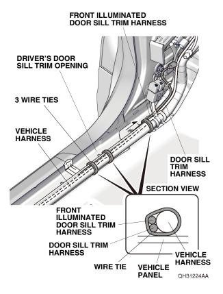
55. Plug the door sill trim harness 2-pin connector into the front illuminated door sill trim harness 2-pin connector.
