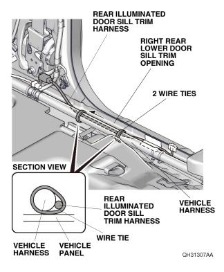
68. Plug the door sill trim harness 2-pin connector into the rear illuminated door sill trim harness 2-pin connector, and secure the 2-pin connectors and door sill trim harness to the vehicle harness with three wire ties as shown.
