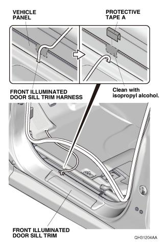
24. Install the protective clip to the protective tape A on the vehicle panel.
