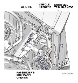
60. Bundle up the excess other accessory harness, and secure it and the 2-pin connectors to the vehicle harness with two wire ties as shown. Go to step 63.
