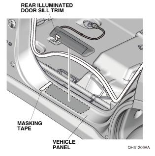
31. While applying light pressure against the rear illuminated door sill trim, carefully remove the taped adhesive backing.
