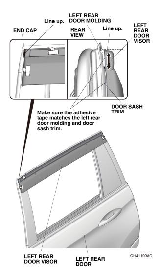
23. While lining up the left rear door visor with the left rear door, apply light pressure against the left rear door visor as shown.
