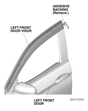
14. Using a rubber roller, apply firm pressure against the left front door visor and roll from one end to the other. NOTE: Apply firm pressure, especially at the ends.
