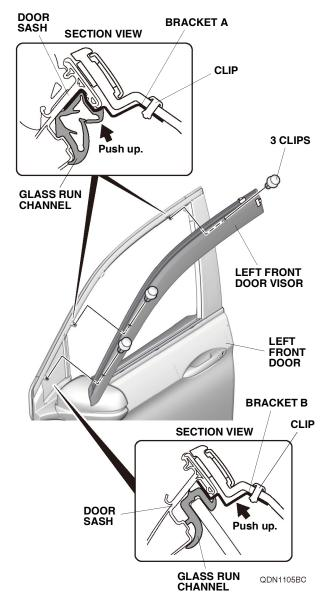
8. Using the three clips, secure the left front door visor to the two brackets A and one bracket B as shown. Make sure to push up on the two brackets A and one bracket B while installing three clips.
