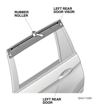
While applying light pressure against the left rear door visor, carefully remove the taped adhesive backings.
