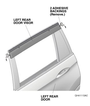
27. Using a rubber roller, apply firm pressure against the left rear door visor and roll from one end to the other. NOTE: Apply firm pressure, especially at the ends.
