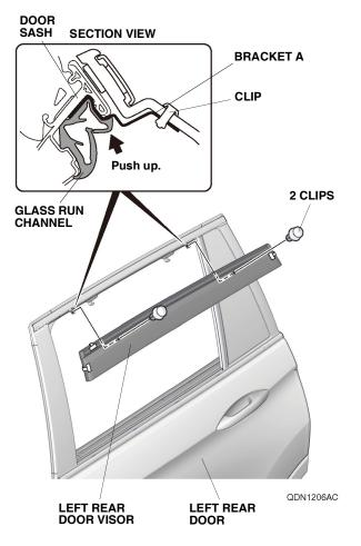
21. Using the two clips, secure the left rear door visor to the two brackets A as shown. Make sure to push up on the two brackets A while installing the two clips. NOTE: Be extremely careful when installing the clips; they cannot be reinstalled after installation. 22. Open the left front door. Line up the left rear door visor as shown.
