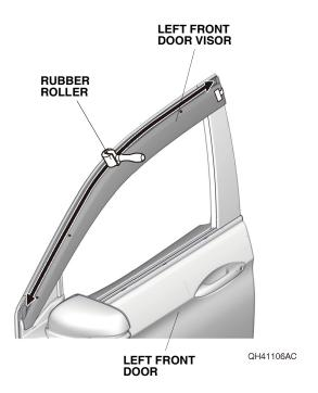
While applying light pressure against the left front door visor, carefully remove the taped adhesive backing.
