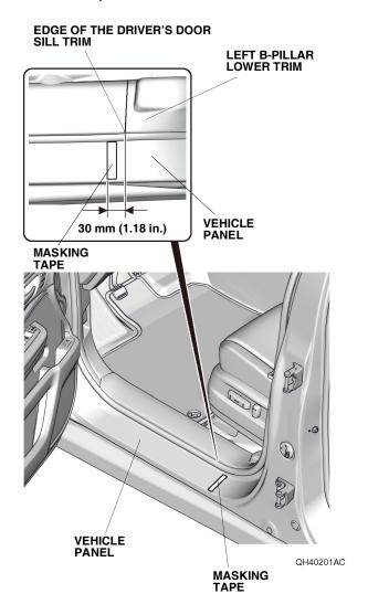
Using the alcohol wipe, thoroughly clean the vehicle panel where the left front door sill protection film will attach.
