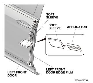
Slowly remove the protective film from the left front door edge film.
