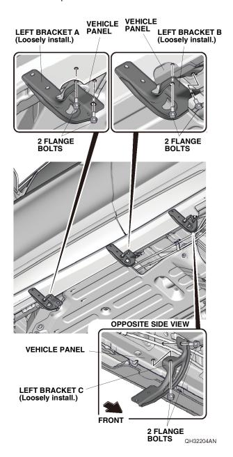
4. With the help of an assistant, install the left running board to the left bracket A, left bracket B, and left bracket C with six flange bolts. Torque the flange bolts to 20 lb-ft (27 N·m).
