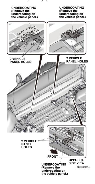
Loosely install the left bracket A, left bracket B, and left bracket C to the vehicle panel with six flange holts
