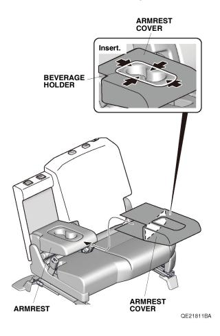
Raise the armrest. Pull out the armrest cover between the armrest and left second row seat-back, and secure the armrest cover with the fasteners.
