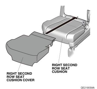
6. Secure the three hooks and fasteners to the right second row seat cushion. Insert one tab to the right second row seat cushion.
