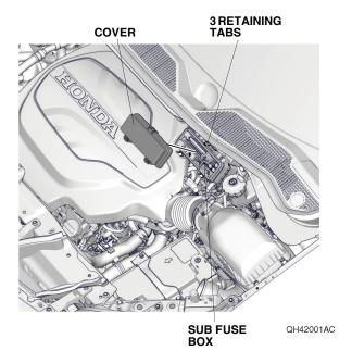
42. Plug the two 20A blade fuses and the 30A block fuse into the sub fuse box.
