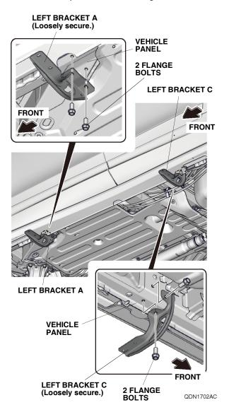
4. Secure the left running board to the left bracket A and left bracket C with four flange bolts. Torque the flange bolts to 20 lb-ft (27 N·m).
