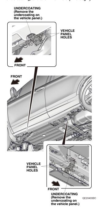
3. Loosely secure the left bracket A and left bracket C to the vehicle panel with four flange bolts.
