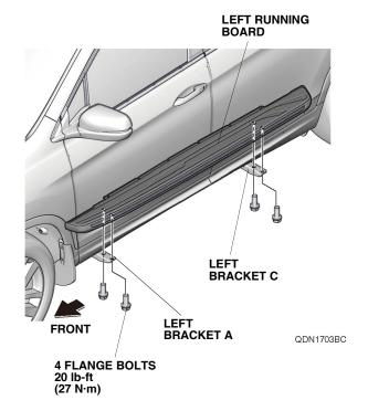
5. Tighten the four flange bolts loosely installed in step 3. Torque the flange bolts to 20 lb-ft (27 N·m).
