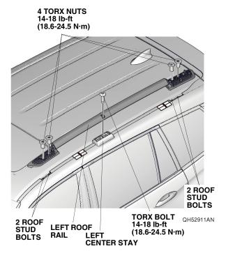
Secure the left roof rail to the left center stay with one TORX bolt. Torque the TORX bolt to 14-18 lb-ft (18.6-24.5 N·m). 16. Install the left roof rail cap to the left roof rail with three retaining tabs.
