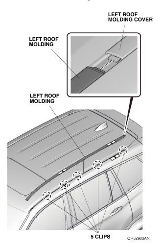
5. Remove the five clips from either the molding or the roof stud bolts.
