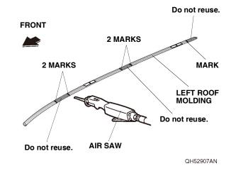
Install the new molding clips to the left roof moldings as shown.
