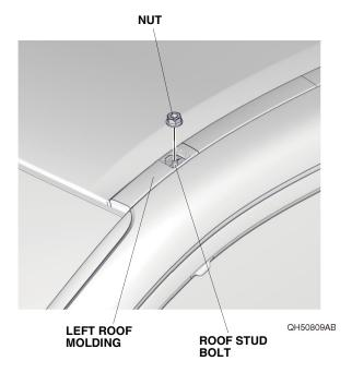
4. Remove the left roof molding as shown.
