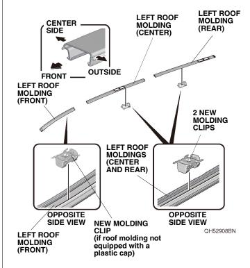
Install the left roof moldings with molding clips. Line up the marks on the four pieces of masking tape made in step 1 on the vehicle panel and left roof moldings.
