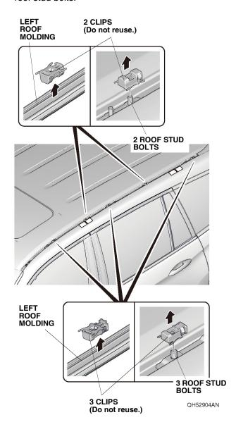
6. Using a putty knife, remove any excess sealant from the six roof stud bolts.
