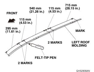
8. While wearing eye protection, use an air saw to cut the molding at the five marks made in step 7. Remove any burrs.
