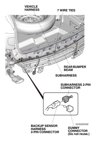
34. Route the subharness, and secure it to the vehicle harness with seven wire ties. With the help of an assistant, install the rear bumper.
