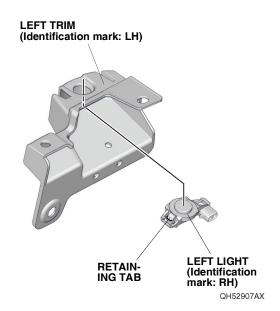
39. Install the left retainer to the left trim with one self-tapping screw.
