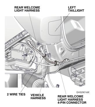
If the vehicle is equipped with the accessory trailer harness, go to step 24; otherwise, continue with step 22.
