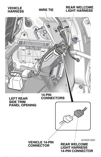
28. Secure the rear welcome light harness and 14-pin connectors to the vehicle harness with one wire tie.
