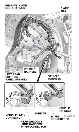
23. Secure the rear welcome light harness and 14-pin connectors to the vehicle harness with four wire ties as shown. Go to step 29.
