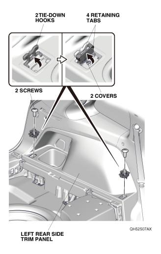
9. Using a plastic trim tool, pull the cover, and remove the cargo hook.
