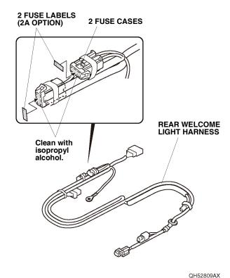
19. Remove the vehicle grommet. Route the rear welcome light harness through the vehicle panel hole as shown.
