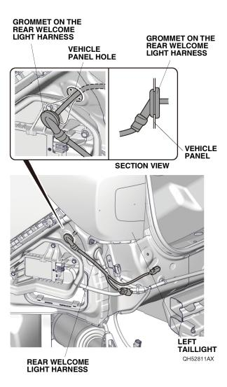
21. Secure the rear welcome light harness and rear welcome light harness 4-pin connector to the vehicle harness with two wire ties as shown.
