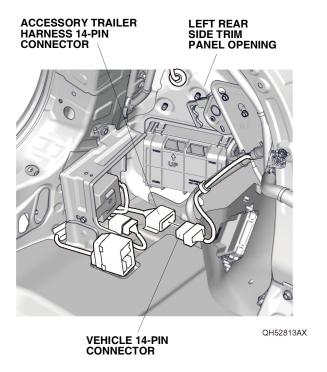
25. Remove the tape to free the rear welcome light harness 14-pin connector. Route the rear welcome light harness along the vehicle harness, and plug the rear welcome light harness 14-pin connector into the accessory trailer harness 14-pin connector.
