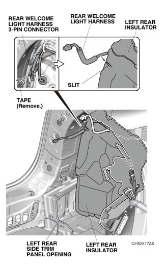
31. Plug the rear welcome light harness 3-pin connector into the accessory hands-free access power tailgate switch. Install the left rear side trim panel.
