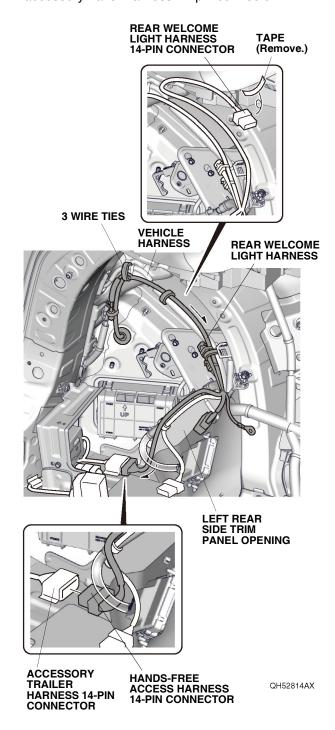
26. Secure the rear welcome light harness to the vehicle harness with three wire ties.
