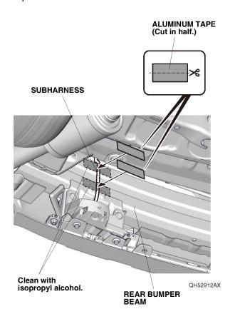
45. Using scissors, cut one piece of aluminum tape in half, and secure the subharness to the rear bumper beam with two pieces of aluminum tape as shown.
