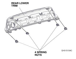
13. Install the rear lower trim to the rear bumper with eight retaining tabs and four bolts removed in step 8. Then, plug the vehicle connector to the hands-free access unit connector (if equipped).
