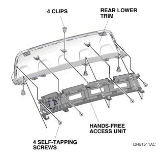
12. Install the four spring nuts removed in step 9 to the rear lower trim.
