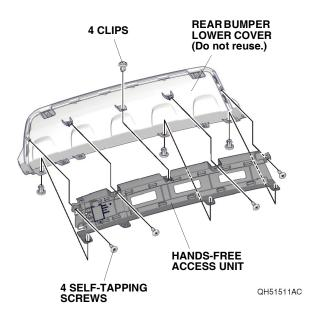
11. Install the hands-free access unit to the rear lower trim with four clips and four self-tapping screws removed in step 10.
