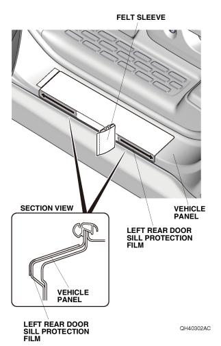
21. Using a shop towel, wipe off the 3M protective tape application solution. Allow the left rear door sill protection film to dry thoroughly. Remove the masking tape.
