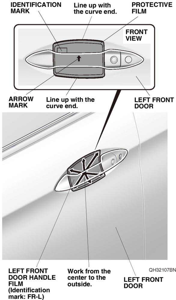
6. Starting from the center and working outward, use the mini soft spreader/applicator to smooth out the left front door handle film. If you see an air bubble, stop and gently peel up that section to work out the bubble. Work slowly and keep pressure against the left front door handle film.
