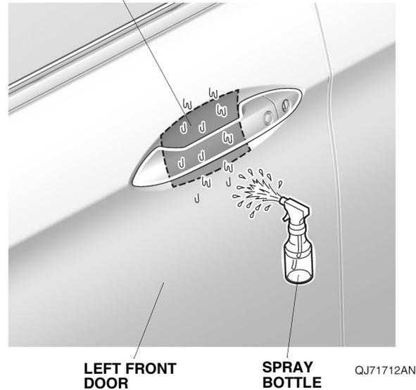
3. Remove the adhesive backing from the left front door handle film.
