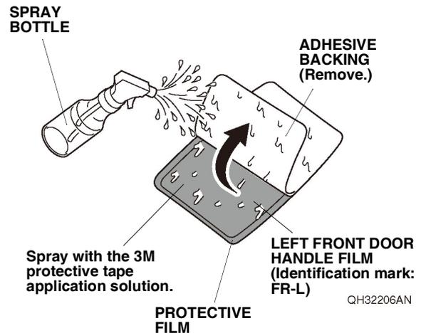
4. Spray the left front door handle film and protective film with the 3M protective tape application solution.
